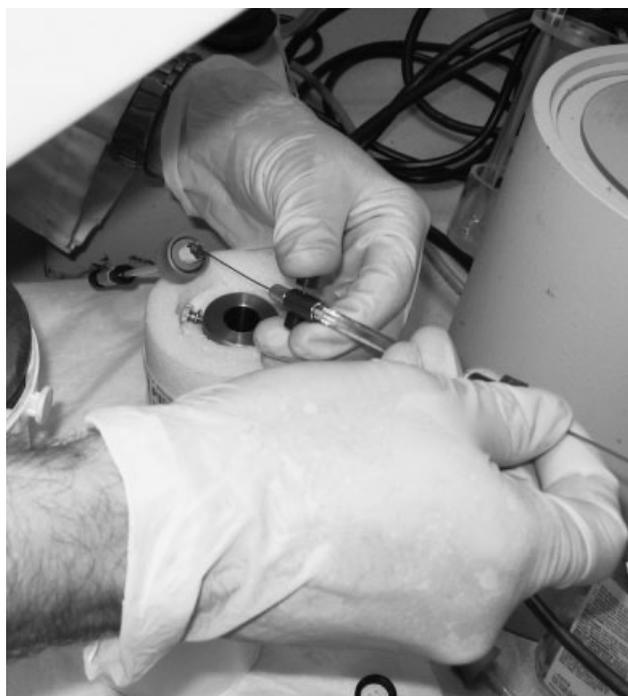
**Figure 4.** Dosing of a cigarette with [<sup>11</sup>C]nicotine. The microliter syringe, technique of loading on the cigarette fragment face, the fragment itself and holder, and the tubing attached to the vacuum source for drying, which subsequently is attached to the smoking apparatus, are all shown.
